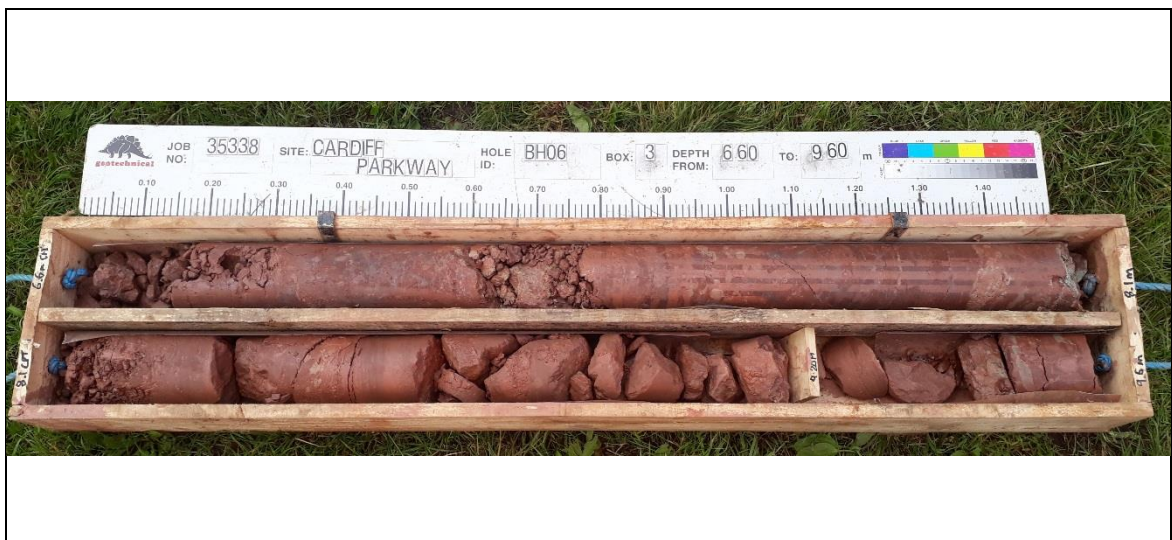
Borehole: BH06 Box 3: 6.60-9.60m
