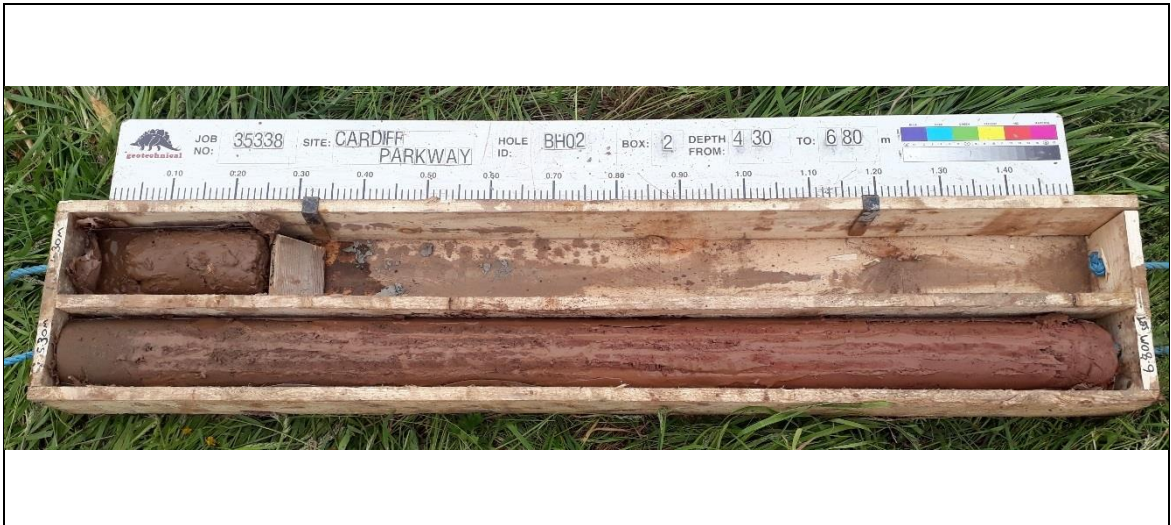
Borehole: BH02 Box 2: 4.30-6.80m
