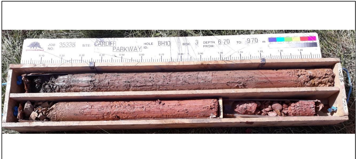
Borehole: BH10 Box 3: 6.70-9.70m
