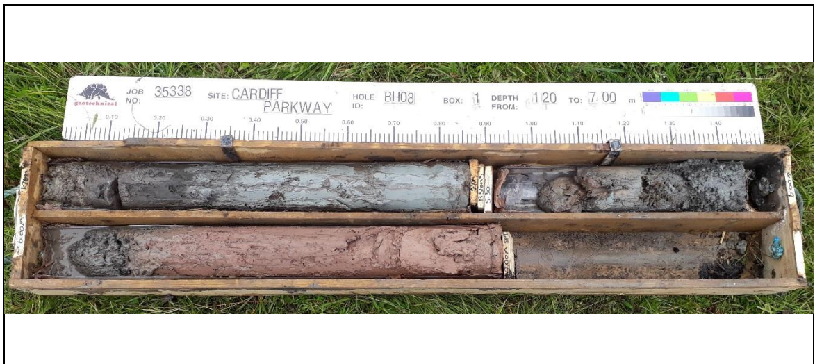
Borehole: BH08 Box 1 1.20-7.00m
