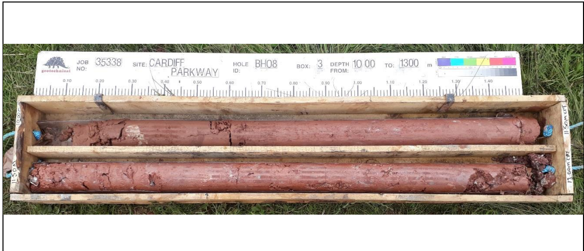
Borehole: BH08 Box 3 10.00-13.00m
