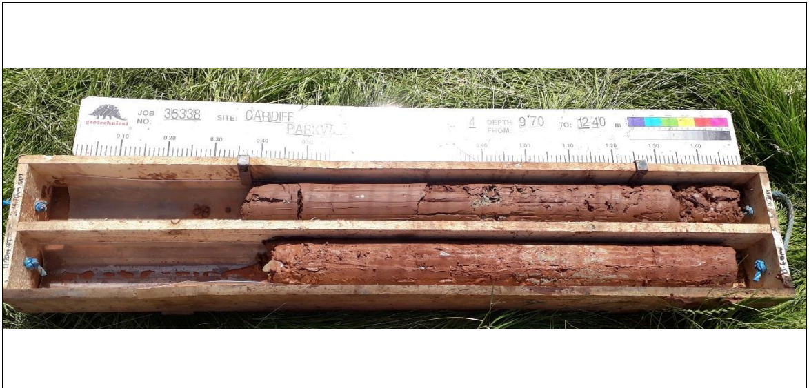
Borehole: BH11 Box 4: 9.70-12.40m
