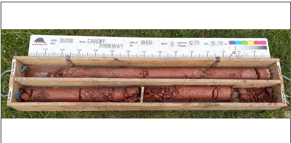
Borehole: BH05 Box 5: 12.70-15.70m
