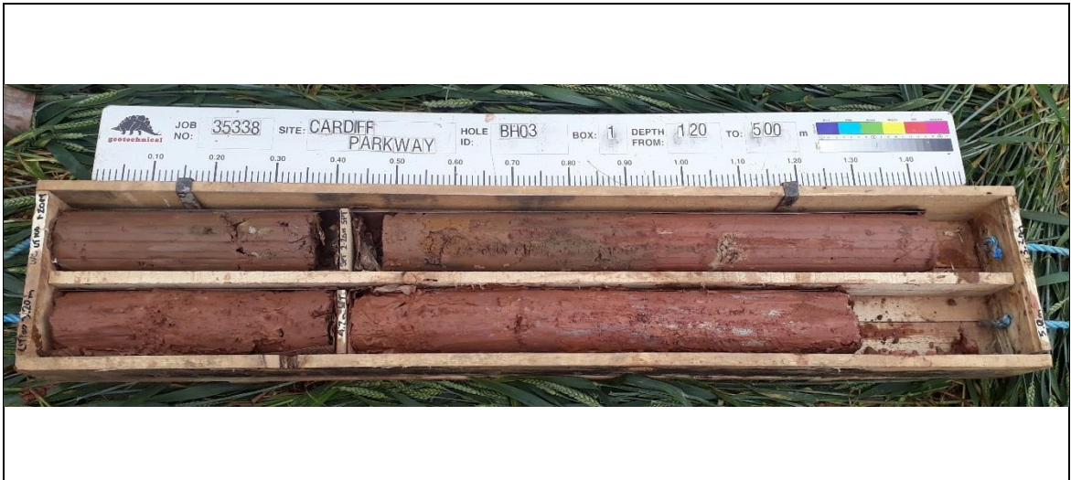
Borehole: BH03 Box 1: 1.20-5.00m
