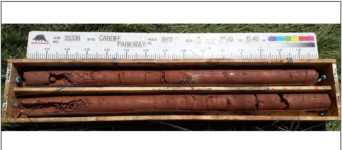
Borehole: BH11 Box 5: 12.40-15.40m
