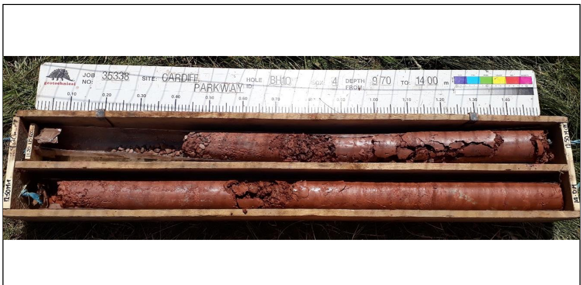
Borehole: BH10 Box 4: 9.70-14.00m
