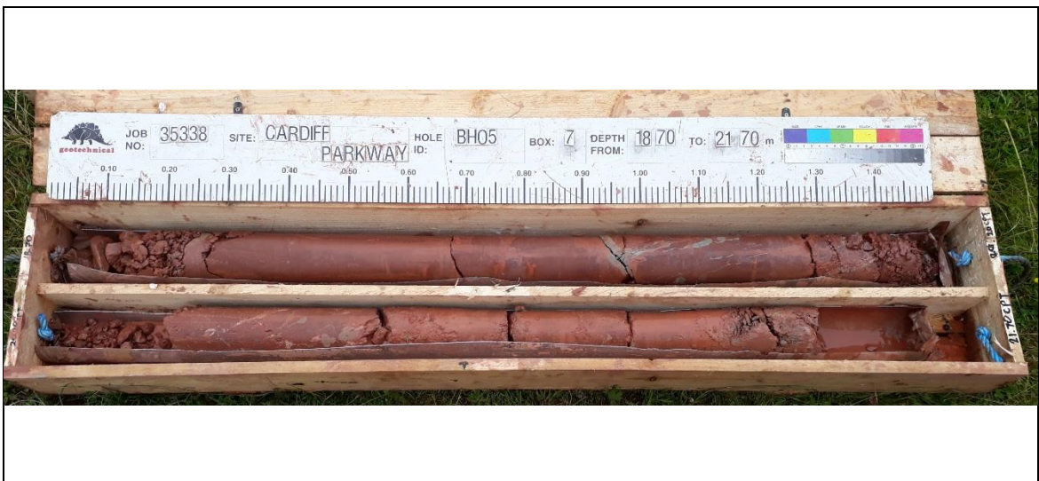
Borehole: BH05 Box 7: 18.70-21.70m
