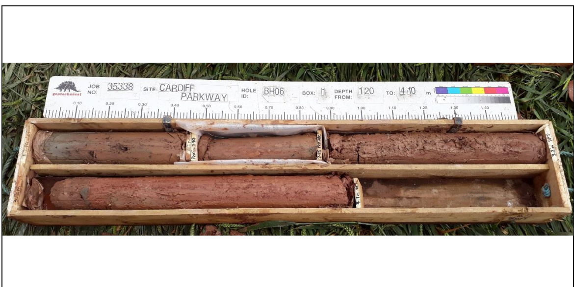
Borehole: BH06 Box 1: 1.20-4.10m
